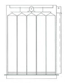
The dust house is equipped with either an air powered or electric powered vibrator used for cleaning of the bags. If air powered, connect air supply line to the 3/8" NPT coupling located on center above the door, and supply the vibrator with 80 psi oiled or non-oiled air. If electric powered, reconnect power cord which exits the top side of dust house to the control box supplied. Operate vibrator for approx. 10-15 minutes after each load of material has been blown in.
